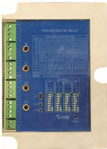
The PSW Self-powered protection device is a kind of protection device for 10 kV feeder lines which has over current, instantaneous trip and ground protection functions. This product can be used in conjunction with the ONT-W series current transformers (CT), and the power is supplied from line current through CT, so over current, instantaneous trip and ground protection for distribution network lines could be achieved without auxiliary power supplies by driving low power trip coils.
