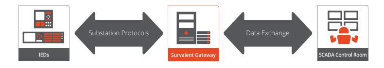
Interoperability is achieved in the data exchange by defining servers, virtual RTUs, and datasets. The server editor allows you to define links to other systems. For each link, you specify the type of interface, the communications ports or IP address used to access the other system, and communication parameters.
